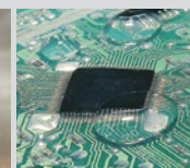
A resin-potted circuit board
